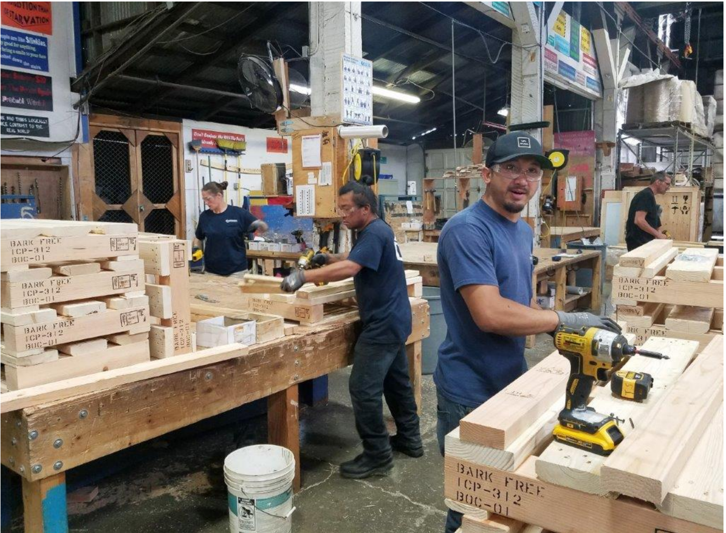
CREW BUILDING SMALL HEAVY DUTY SKIDS AT ICP SHOP
